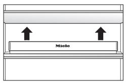
Pull the active charcoal filter holder upwards to remove it from the shelf.
